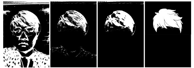
Figure 7. The hair segmentation used in hair matching is created via a combination of masks. Left: The frequency mask and color mask generated through thresholding. Right: The morphologically opened hair segmentation and binary mask of the best matching anime hair.
